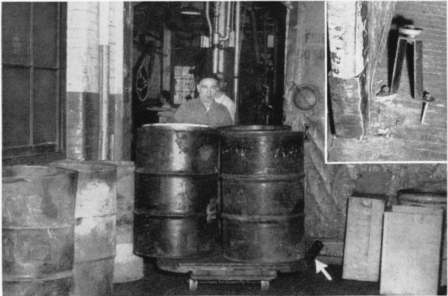
In the photo at the right, Joseph Daddona (Truckers) poses with a barrel truck at one of these tight spots to show how aisle congestion causes delay and property damage. Arrow points to the fire door guide which had been broken sometime before the picture was taken.
